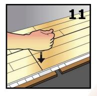
11. By pressing the board at the end, the tongue will yield and "lock" the boards together.
